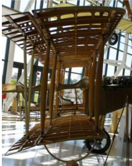
*This display of a 1917 Curtiss Jenny shows the wooden internal structure of the aircraft.*
